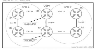
An architect must design a solution that uses the direct link between R1 and R2 for traffic from 10.10.10.0/24 toward network 10.10.20.0/24. Which solution should the architect include in the design?
